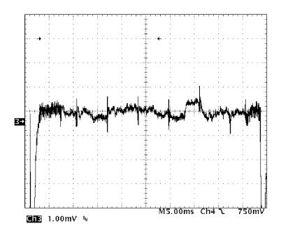
Figure 4-1: Properly adjusted frequency response
