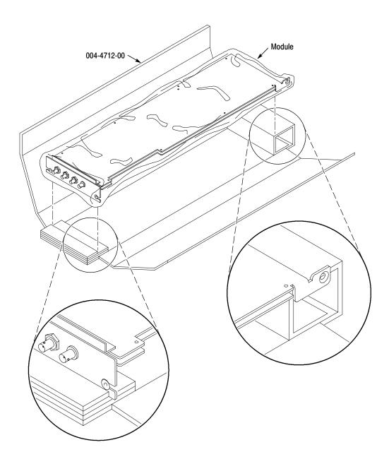
Figure 6-1: Placing the module in the protective wrapping
