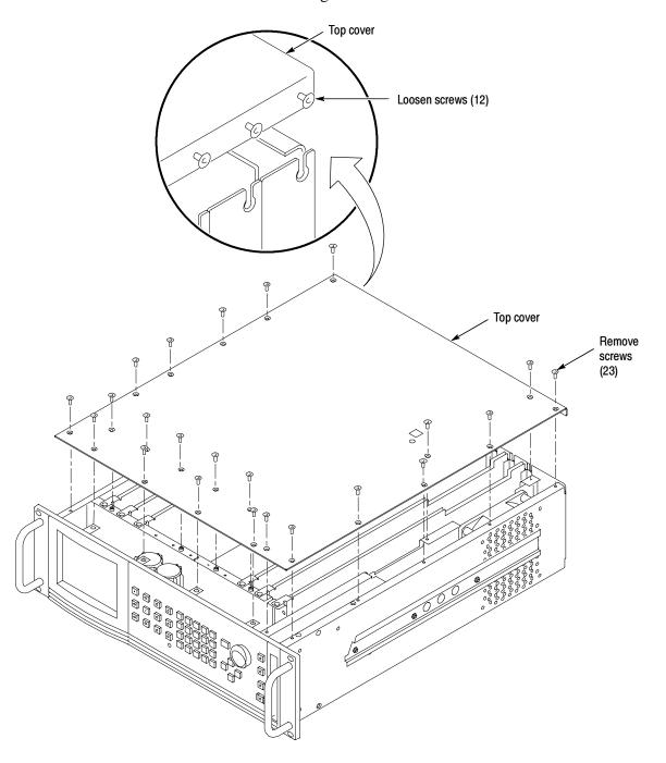
Figure 2-2: Top cover removal
