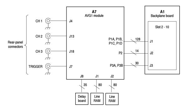
Figure 9-1: AVG1 module connections
