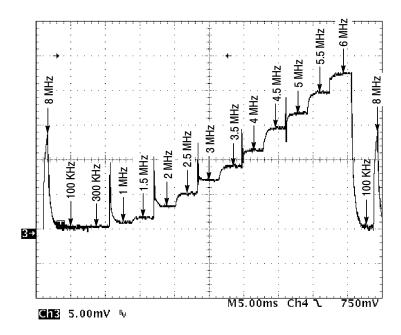
Figure 4-2: Poorly adjusted frequency response
