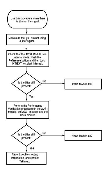
Figure 6-12: Flowchart for jitter on signal
