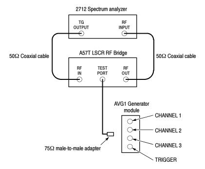
Figure 4-3: Equipment hookup for checking return loss
