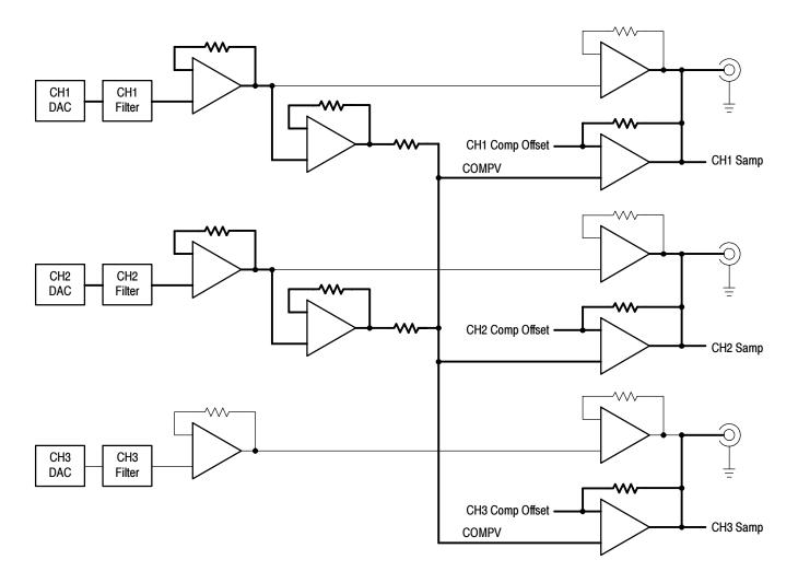
Figure 3-2: Hardware modulated signal mode (three channel composite)
