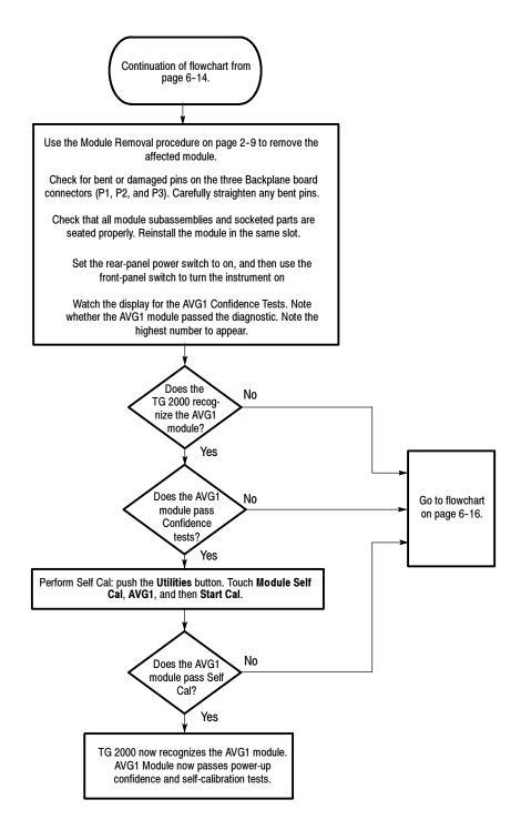
Figure 6-5: Flowchart for checking the current module installation slot
