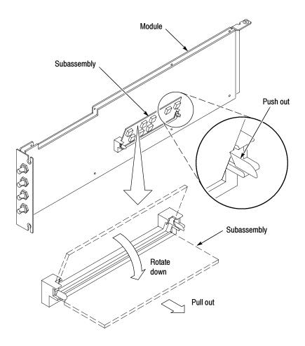
Figure 6-3: Removing a subassembly from a module
