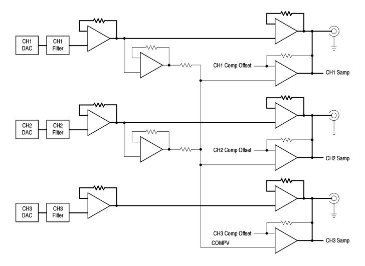
Figure 3-4: Component and software modulated signal mode
