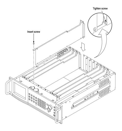
Figure 2-5: Installing the module
