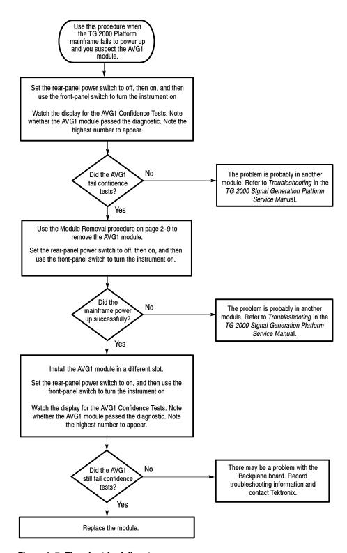
Figure 6-7: Flowchart for failure to power up
