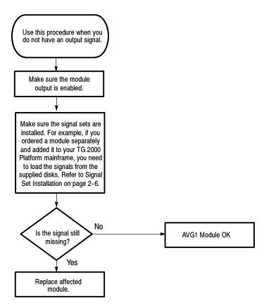
Figure 6-11: Flowchart for missing output signal
