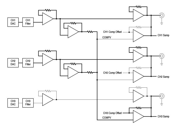
Figure 3-3: Hardware modulated signal mode (YC composite)
