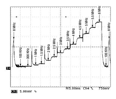
Figure 5-3: Poorly adjusted frequency response
