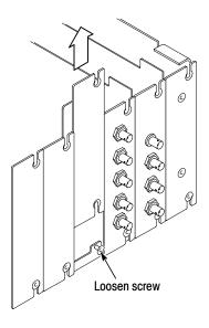
Figure 2-3: Removing the rear panel
