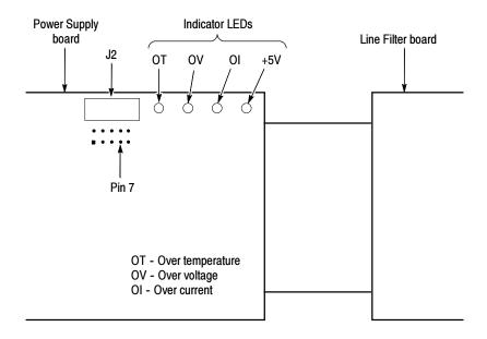
Figure 6-9: Measuring the battery charging circuit
