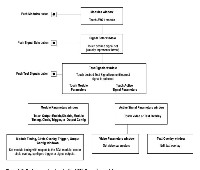
Figure 2-7: Basic menu structure for the AVG1 Generator module
