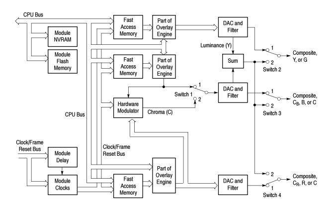
Figure 3-1: Simplified block diagram of the AVG1 Analog Video Generator module
